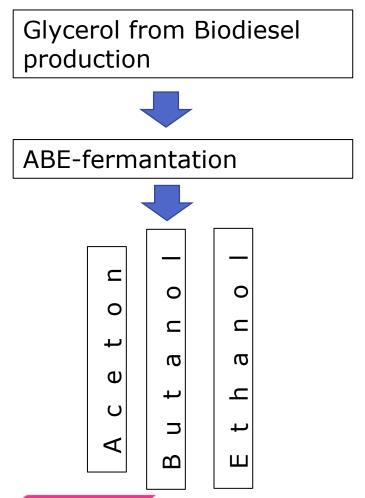
Carbohydrate-based waste streams are used as raw material, from which three main products are produced through the fermentation reaction:
